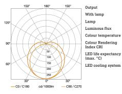
9 W Yes, STEINEL LED system LED cannot be replaced 595 lm ure 3000 K g 80-89 ncy 50000 h em Passive Thermo Control
